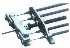
Install equaliser bar as pictured. M12 threaded rod must protrude 100mm behind equaliser chassis bracket as pictured.
