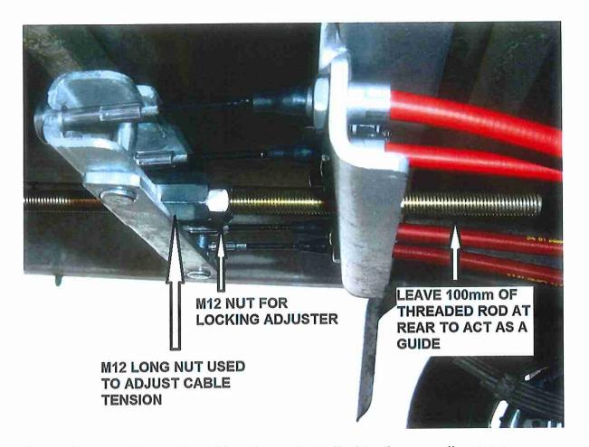
Once the coupling pull rod has been installed to the equaliser, as pictured above, pull the hand brake lever on 3 to 4 times to settle it all into its working position.
