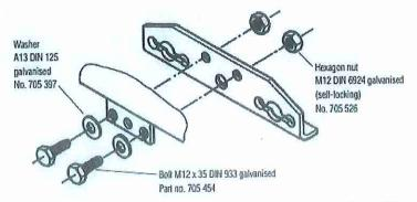
Cable equaliser chassis bracket is to be installed no more than 500mm in front of the centreline of front axle.
