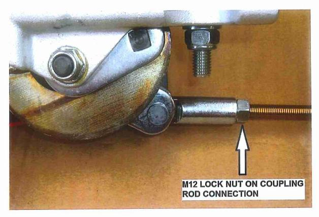
The brake actuation pull rod connection on the Euro 35 coupling is internally threaded M12x1.75. It is recommended that Grade 8.8 M12 threaded rod be used at each end of the brake pull rod, with the centre section of plain M12 pull rod being of equal grade and quality.
