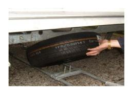
Take out the security chain pin and unfasten the plastic nut of the AL-KO spare wheel carrier. Slide it out to its full extent and remove the replacement wheel. Slide the AL-KO spare wheel carrier back into position and refasten the black plastic nut and security chain pin.
