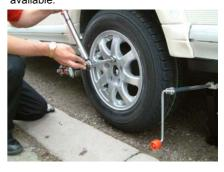
Locate the replacement wheel onto the brake drum and fasten wheel bolts finger tight. Using an AL-KO torque wrench, torque up the wheel bolts to 88Nm or 65lbs/sqft in the correct sequence. I.e. North, South, East and West. Remove the axles stand (if used), raise the corner steadies, raise jockey wheel and release the handbrake.
