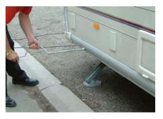
Use the AL-KO corner steady brace to lower the corner steadies on the same side as the wheel to be changed. This is to assist stability of the raised caravan. DO NOT use the corner steadies to jack up the caravan. For additional safety we recommend the use of an axle stand, if available.
