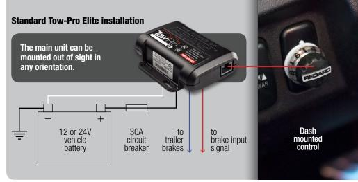
The remote head control is mounted in the dash of your vehicle and the electronic module is mounted out of sight, making the Tow-Pro Elite ideal for vehicles fitted with knee or lower leg airbags.
