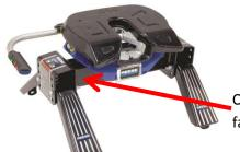
Once completed, the label should be affixed to the hitch on the vertical side face of the cross beam, facing rearwards, when the hitch is on the vehicle.
