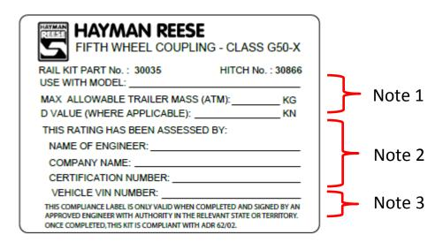
**Note 1**: This information is assessed by the Approved Engineer. The D Value rating MUST be shown for tow ratings between 3500 Kg and 4500 Kg. The words "Use with Model" are specified in ADR 62/02. For further guidance on this, please refer to ADR 62/02.
