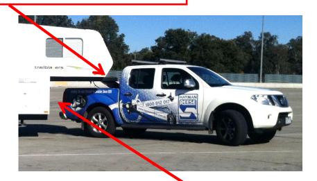
Also consider the clearance between the front skirt of the caravan and the rear corner of the vehicle (and also the tailgate when down) where applicable.
