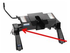
Once completed, the label should be affixed to the hitch on the vertical side face of the cross beam, facing rearwards, when the hitch is on the vehicle.
