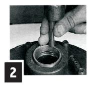
Use cup driver or mild steel bar to solidly seated against rotor hub cup surfaces. Never use a cone to drive a cup.
