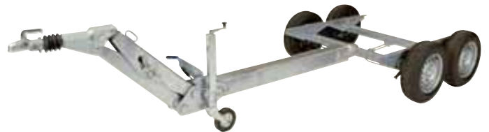
Tandem chassis with adjustable height connection assembly
