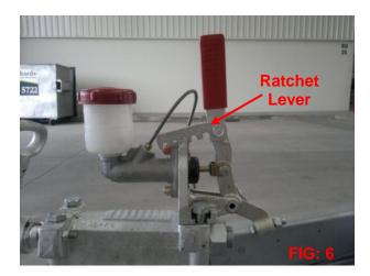
Before disconnecting the Trailer from the Tow vehicle apply the Park Brake
