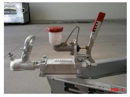
Override Coupling & Hydraulic Conversion Fitted
