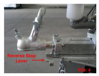
When reversing still with coupling properly connected onto tow vehicle & safety chains fitted, Ensure
