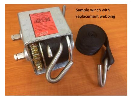
The first step is to fully unwind the winch webbing to expose the drum core and roll pin that holds the shaft in place.
