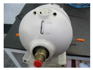
Remove the brake fluid reservoir cap.
