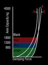
The Hysteresis Diagram (left) demonstrates the improved damping performance provided by the AL-KO Octagon Shock Absorber on a single axle chassis.
