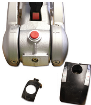
Fig 18 Cheese-head screw revealed
