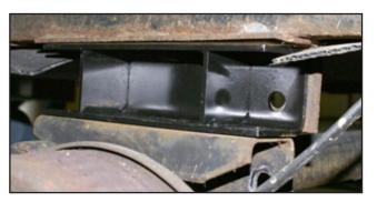
4. Install the two (2) bolts through the back of the spacer and the frame bracket. Each bolt requires one (1) washer on the nut side only. Install the other two (2) bolts through the bottom of the spacer securing it to the axle bracket.
