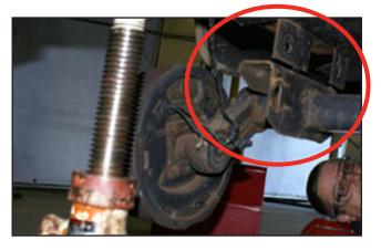
3. Place the spacer between the frame and the axle mounting bracket. The spacer should be installed with the open side away from the side mount hanger.
